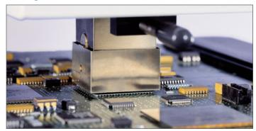
Newly designed reflow head provides smooth, precise movement with no drift, allowing for repeatable and accurate placement.
