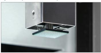
New Vacuum Pick design is more robust, utilizes an optical sensor, is counterweight balanced, and uses precision high temperature linear ball bearings for the highest sensitivity in placement and pick-up.
