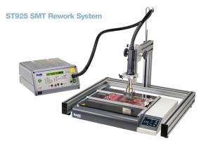
The ST925 combines three popular PACE products together into one convenient, low-cost SMT Rework System. The system is comprised of the ST325 Programmable Convective/Hot Air Rework Station, the PH100 Low Profile Infrared Preheater, and ST500A Z-Axis Platform. Together, the system provides a powerful 575 Watt convective top-side heater plus a 1600 Watt IR bottom-side preheater which allows operators to safely rework PCBs.
