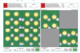
Quad-Field Imaging allows up to *four corners* of a large component (and its pads) to be viewed under high magnification, providing perfect alignment of outsized BGAs or fine-pitch QFPs.
