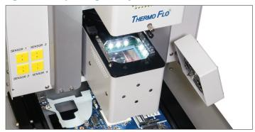
An automated Vision Overlay System uses a dichroic beam-splitting prism, high intensity LEDs, and new high definition 1080p camera to easily align any component.
