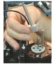
6. Before installing the Theta Knob Assembly, be sure to properly line up the Vacuum Pick Control Knobs.
