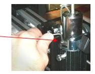
4. Carefully lift the Pick Shroud from the Reflow Head Assembly.
