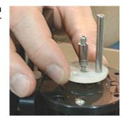
5. Insert the Manifold Vacuum Assembly and tighten the vacuum pick with a 7/32" open-end wrench. Must be snug but do not over tighten!
