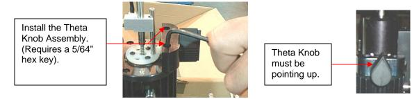
**NOTE:** It is also possible to adjust the Theta Knob by adjusting its position on the shaft. This will require a 5/64" hex key to loosen the two setscrews.
