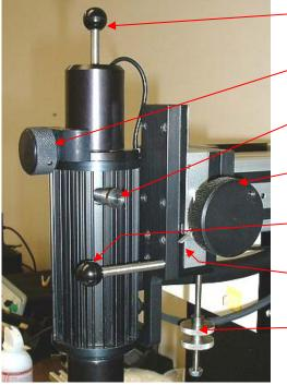
Vacuum Pick Plunger Knob Theta Control Knob Vacuum Pick Height Adjustment Control Knob **Z-Axis Control Knob Reflow Head Rail Knob** Z-Stage Lock **Reflow Head Repeatable Down Stop**
