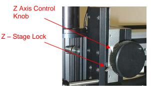
be adjusted unless there is a problem with the reflow head drifting or if the reflow head is too difficult to move with the Z axis control knob. Do not over tighten Z-Stage Lock. A properly adjusted Z-Stage lock will allow the Z Axis Control Knob to move to any position without slipping.
